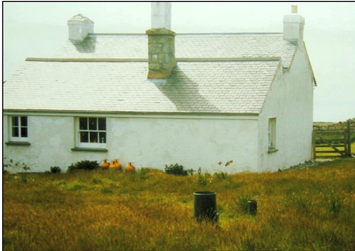
Plate 3: The two rain gauges in the top paddock of Stoneycroft. The smaller gauge is used for daily amounts, and the large gauge records short-period extreme rainfall rates.
