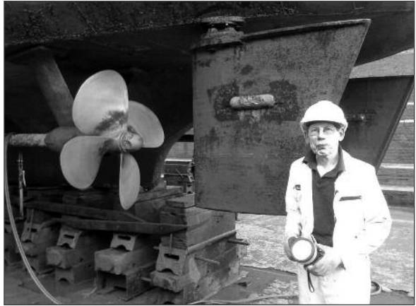
Ship Superintendent Jack Bater inspects Oldenburg's propellers during the annual dry-dock at Sharpness. Photo: Derek Green
