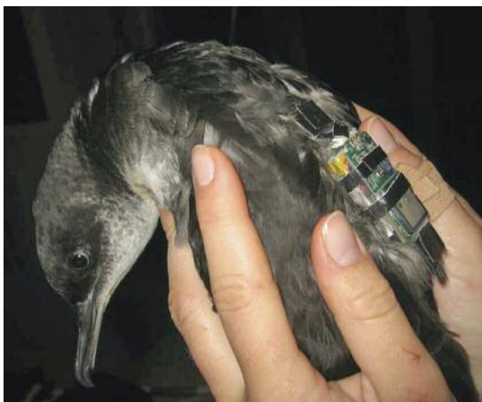
Figure 3. An example GPS attachment. A sealed GPS logging device attached to a bird using TESA tape.
