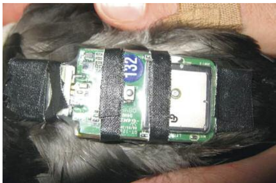
Figure 2. The GPS device is positioned to sit like a backpack above the bird's centre of gravity, leaving the wings completely free to move.
