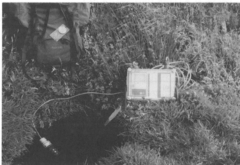
Fig. 2: The pHOX® Type 67 Logging D.O. Temperature meter deployed at one of the sampling stations, St. Mark's Bay Stream (West 2) (Photo: P.S. Long)
